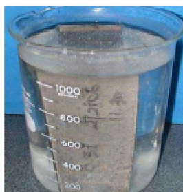
After 1500 hours Mild steel immersed in sea water with 0.05% of Vapro VCI-844
